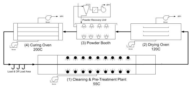
Figure 1.1 Powder Coat Plant Schematic Layout
