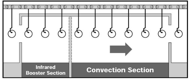
Figure 7.1 convection oven with infrared booster section
