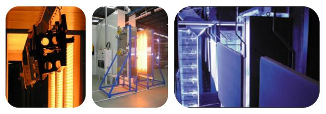
Figure 6.2 from left to right, IR oven, Combined IR/Convection oven and Combined IR/UV oven
