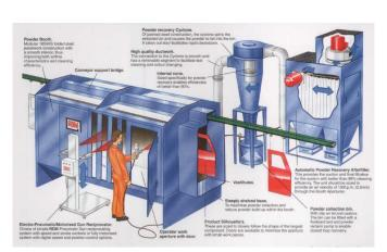
Figure 1.2 Powder Booth Schematic Layout (www. http://rdmengineering.co.uk)
