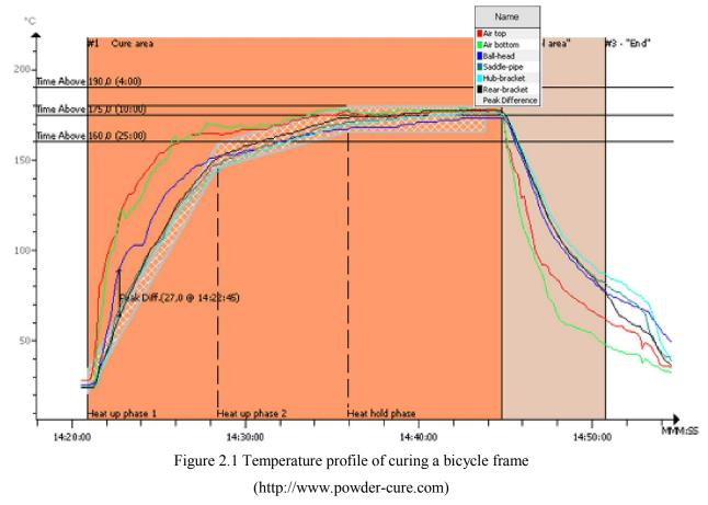
Therefore, the line speed and production rate are limited by cure cycle time but the part can be stayed for longer period than curing time without effect on finishing quality and colour.
