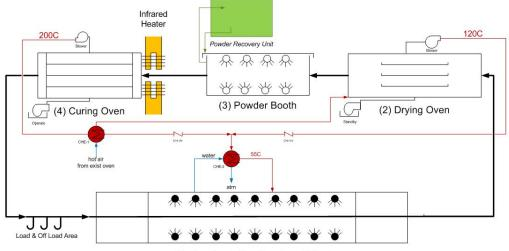
(1) Cleaning & Pre-Treatment Plant Figure 5.1 Conceptual Designs for new Powder Coating Plant
