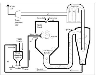
Figure 1.3 Powder Auto-Recycling system, AkzoNobel (1999)
