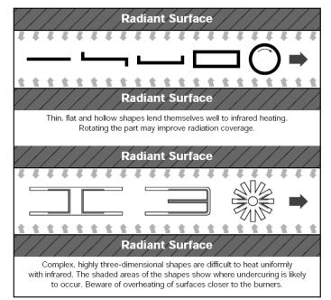
Figure 6.1 Suitable product configurations for IR heating (Eclipes Combustion)
